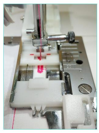
Stitch the buttonhole. The machine should slow down or stop at the end.
