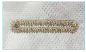
Prior to sewing on your garment, stitch a sample of the style of buttonhole you desire. Adjust the tension, stitch length and width if necessary. Some machines automatically adjust.
